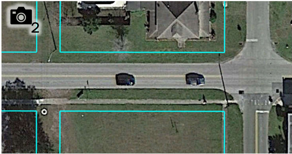
Roadway centerline may need to shift south. A minimum distance from roadway to sidewalk is required in design standards.
