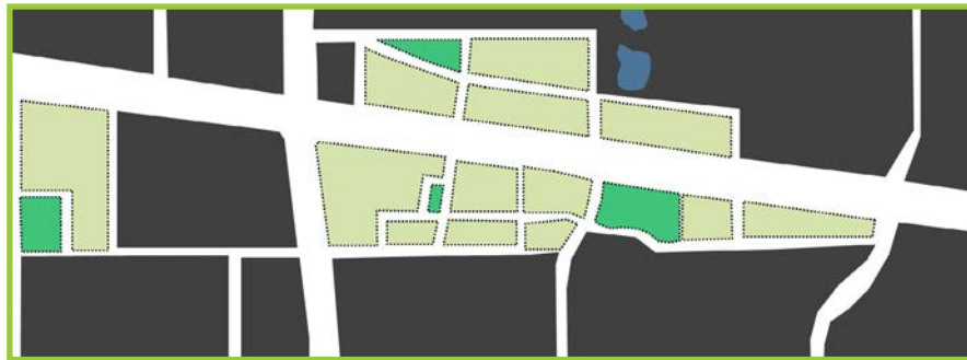
Typical suburban roadway network pattern with large block sizes and few street connections
