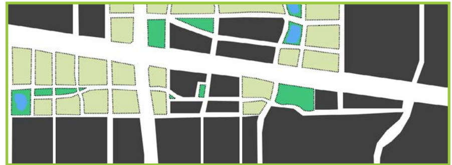
Enhanced street networks disperse vehicular travel along multiple roadways with a number of roadways sharing the load of multi-modal travel
