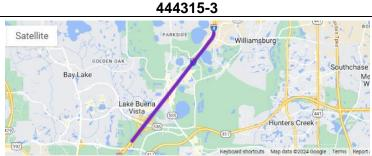
**Description:** The project will construct a single buffer separated express lane on I-4 in the westbound direction from west of State Road (S.R.) 528 to west of Central Florida Parkway. The project will also add the final striping, friction course and tubular markers for the full length of the single buffer express lane on I-4 in the westbound direction from west of S.R. 528 to west of S.R. 536
