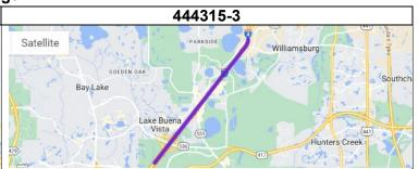
**Description:** The project will construct a single buffer separated express lane on I-4 in the westbound direction from west of State Road (S.R.) 528 to west of Central Florida Parkway. The project will also add the final striping, friction course and tubular markers for the full length of the single buffer express lane on I-4 in the westbound direction from west of S.R. 528 to west of S.R. 536
