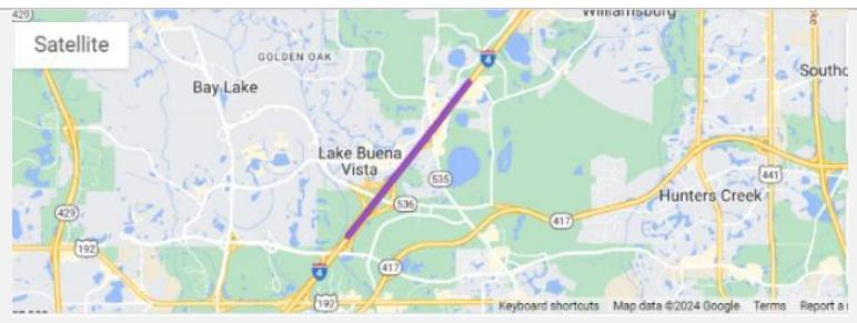
**Description:** This project will add a single, buffer-separated, westbound managed lane to Interstate 4 (I-4) from west of State Road (S.R.) 536 to west of Daryl Carter Parkway. The complete managed lane will be built in three separate projects extending from west of S.R. 536 to west of Sand Lake Road (S.R. 482). The single, buffer-separated express lane will be open once all three segments are completed.
