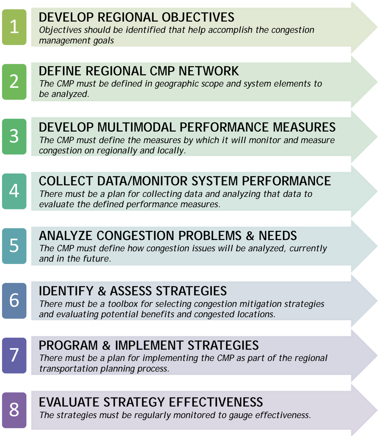
Figure 2-1: Federal Eight-Step Congestion Management Process
