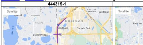
Description: This project will convert the Sand Lake Road and I-4 interchange into a diverging diamond interchange. The Diverging Diamond Interchange (DDI) is a type of interchange in which the two directions of traffic at an interchange cross to the opposite side of
