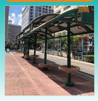
Bus shelters are important for protecting passengers from sun, rain, and other inclement weather, and should be designed with the local climate in mind. Shelters should also have proper lighting and be transparent for the safety and security of passengers. Seating and other amenities, such as trash cans, can also be added for passenger comfort.
