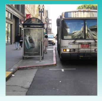
In some areas, where on-street parking is provided, a bus pull-out will be provided for the bus to move out of traffic. An alternative is a bus bulb, where the curb is extended to the travel lane so the bus can pick-up/dropoff passengers without merging in and out of traffic. The additional space can also be used for bus shelters and other amenities.
