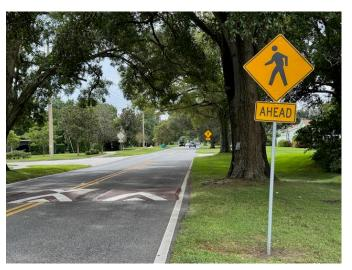
This residential crosswalk near Lake Como School had an average driver yield rate of just **31%** throughout 2024. This year, after the installation of speed humps near the ahead signage leading up to the crosswalk, the driver yield rate doubled to an average of **62%**, demonstrating the effect of reduced vehicular speeds on yielding behavior.
