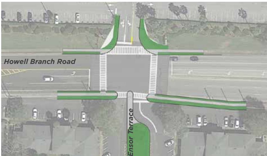
Detail of intersection modifications at Ensor Terrace/Casselberry Commons entrance to decrease pedestrian crossing distances on the north and south legs and construct curb ramps for all crosswalks
