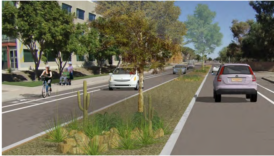
Conceptual Median and Bicycle Lane with Lane Elimination
