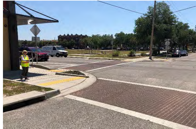
Intersection Bulb-Outs Combined with On-Street Parking and Stamped Asphalt Crosswalk Markings
