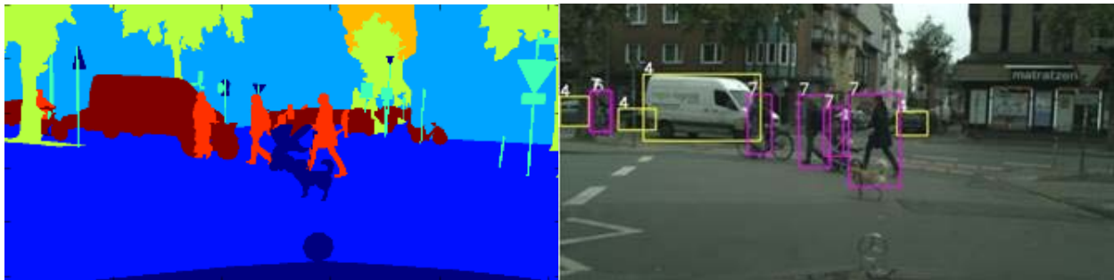
Figure 2: How an Automated Vehicle Senses Objects
