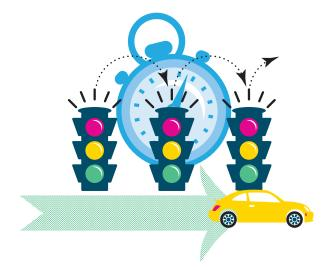
Retiming traffic signals along congested corridors is a relatively low-cost transportation systems management & operations strategy that can result in smoother traffic flow, fuel savings, and reduced vehicle emissions.
