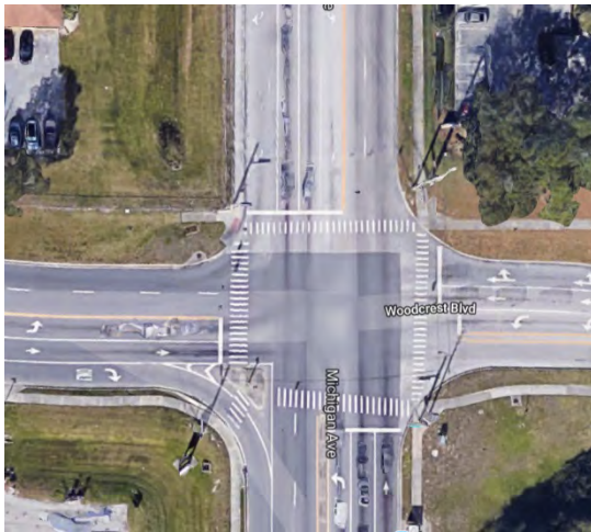
Channelized Right-Turn Lane without Improved Pedestrian Accommodations (not enhanced crosswalk, vehicle acceleration lane present)
