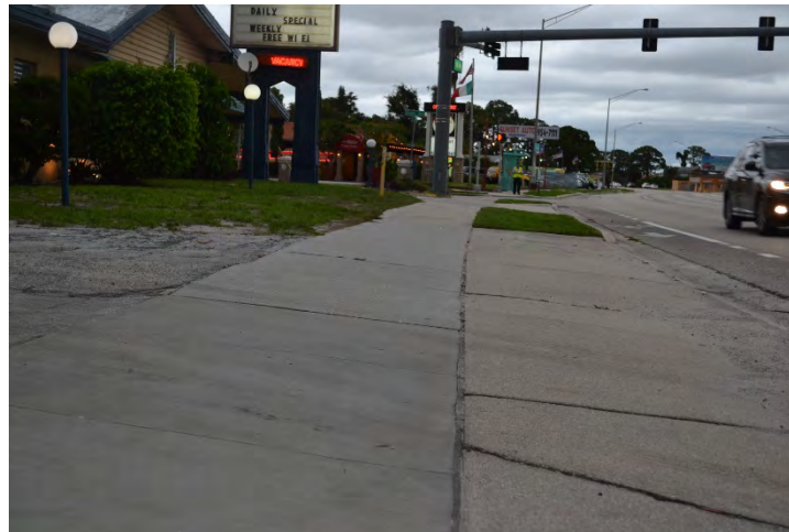
Wide Driveway Entrance with Steep Cross-Slope and Large Turning Radius
