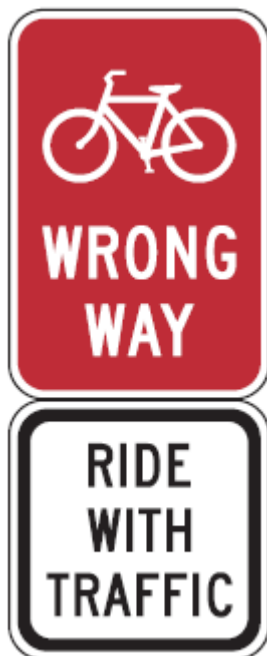
Figure 31 “WRONG WAY” AND “RIDE WITH TRAFFIC” signs (MUTCD, R5-1b (top) and R9-3c (bottom)) 9
