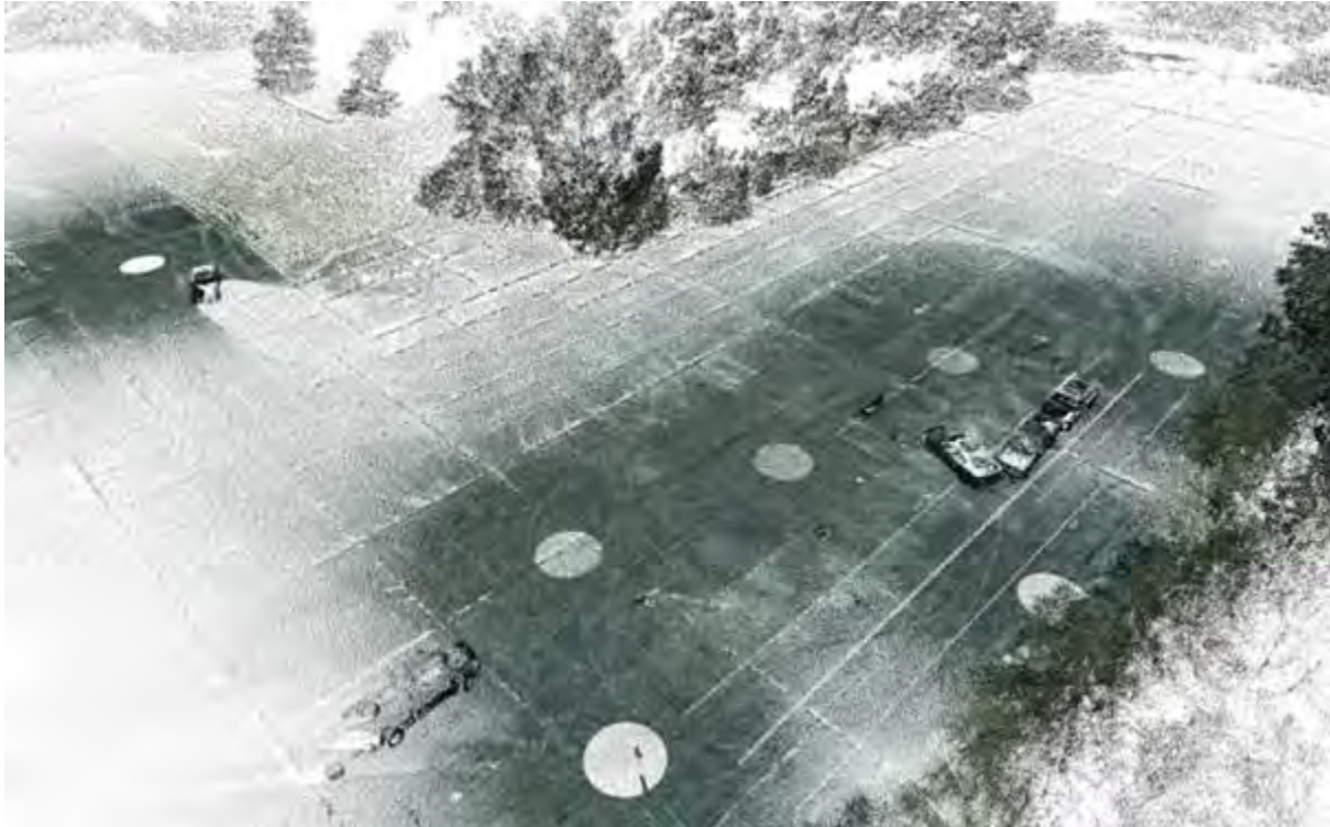
Figure 1: Mock Crash Scene Laser Scanned Imaged by Leica 3D Scanner
