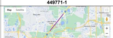
This project will add a single, buffer-separated, westbound managed lane to Interstate 4 (I-4) from west of State Road (S.R.) 536 to west of Daryl Carter Parkway. The complete managed lane will be built in three separate projects extending from west of S.R. 536 to west of Sand Lake Road (S.R. 482). The single, buffer-separated express lane will be open once all three segments are completed.
