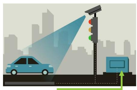
Data from traffic detection systems is sent to the signal cabinet(s) located at each intersection
