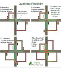
pedestrians; expands grid connectivity; enhances and motivates TOD; often very low cost; easy access to retail; back-side auto access; compatible with traditional signals. Disadvantages: Initial confusion for drivers; resistance when adding traffic to existing residential backway; potential out of direction travel.
